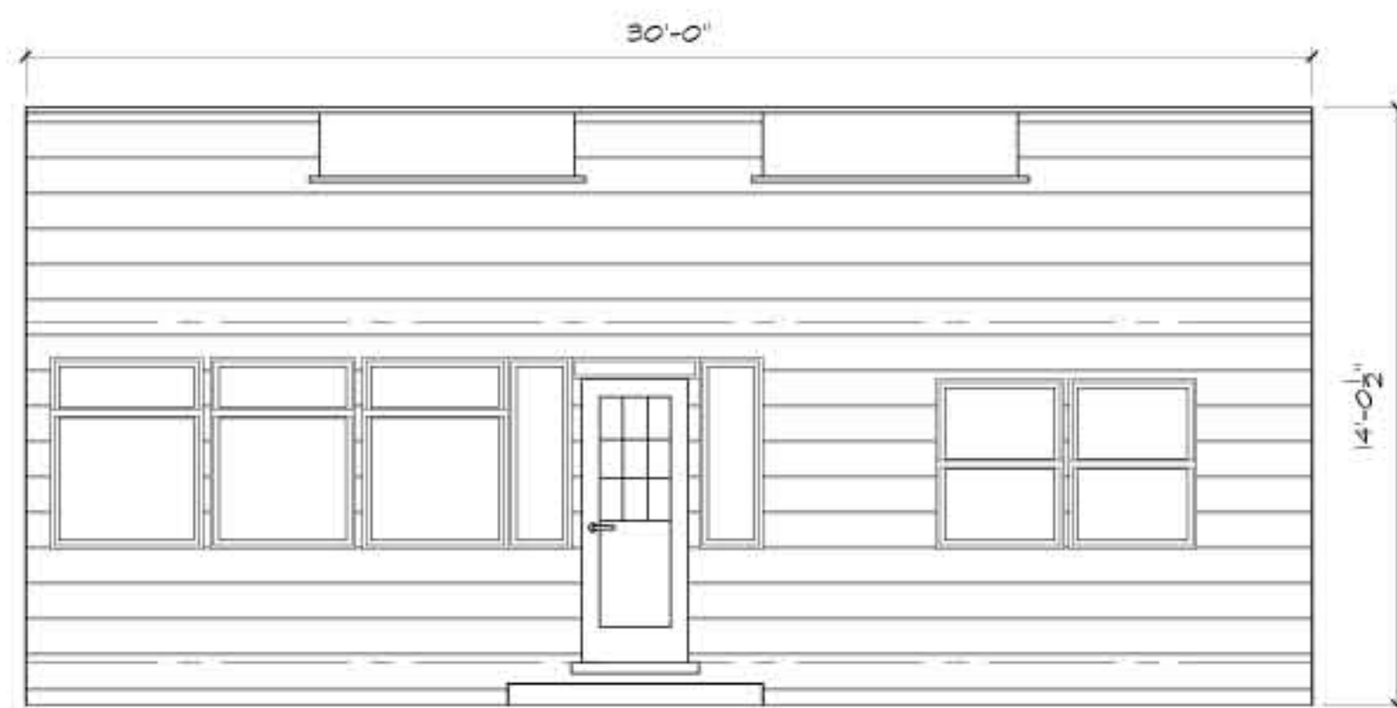
EXISTING NORTHEAST ELEVATION TO REMAIN UNCHANGED SCALE: 1/4"=1'-0"
